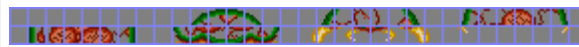
Fig 8.2c: how fig 8.2a should be stored in memory when using 1D mapping.
