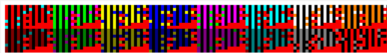
Fig 7.2c: the data of fig 7.2a, interpreted as 4bpp data. If you see something like this (and you will), you now know why.
