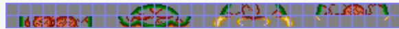
Fig 8.2c: how fig 8.2a should be stored in memory when using 1D mapping.
