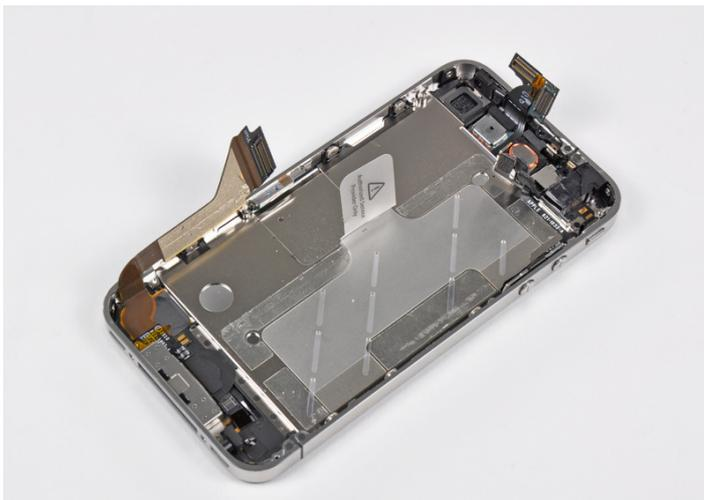
Figure 14: The iPhone 4's integrated UMTS, GSM, GPS, Wi-Fi and Bluetooth antennas on the stainless steel inner frame [15]
