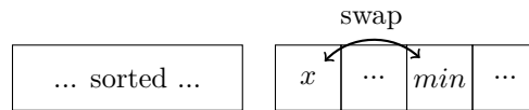
Figure 9.2: The left is sorted, repeatedly find the minimum and swap to the right position.
