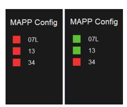
The Missed Approach Configuration Unit automatically appears when you log on any approach/departure, terminal or area radar position (suffix \_APP or \_CTR). It allows you to select which runways you wish to receive missed approach alerts for.
