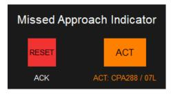
When the missed approach alert is activated, the ACT button flashes bright orange, the RESET button turns on bright red and an aural alert begins playing. Any APP/CTR controller that has chosen to receive alerts for that runway has been alerted. If you wish to cancel the alert before acknowledgement, click the RESET button to reset the indicator back to its original state.
