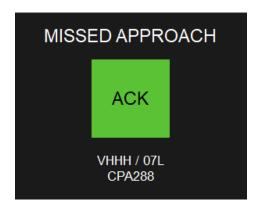
To acknowledge the missed approach, click the flashing orange ACK button once. The ACK button turns green to indicate that your acknowledgement has been sent to the tower controller. At this point, clicking the green ACK button again will dismiss the alert unit.
