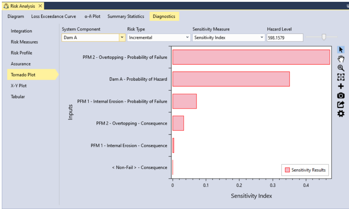
Figure 11. Tornado plot sensitivity diagnostic plot in RMC-TotalRisk.
